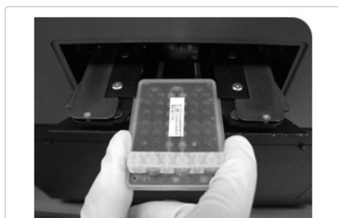
Figure 1: A low cost, fully automated, user-friendly, lab on a chip genotyping analysis system (TPSA-003) predicting the risk of rashes by identifying DNA polymorphism markers (HLA-B*3505) that indicate a high correlation with the risk of drug rash occurrence, which is a side effect of the antiretroviral therapy, nevirapine.
